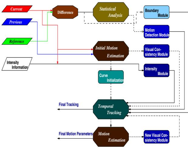
**Figure 1.** Flow chart for motion estimation and tracking.
