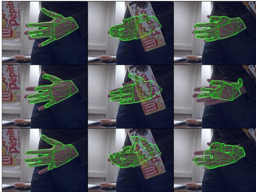
Fig. 7. Tracking results comparisons: each row corresponds, respectively, to the smart particle filter, the classical particle filter and the single hypothesis method.
