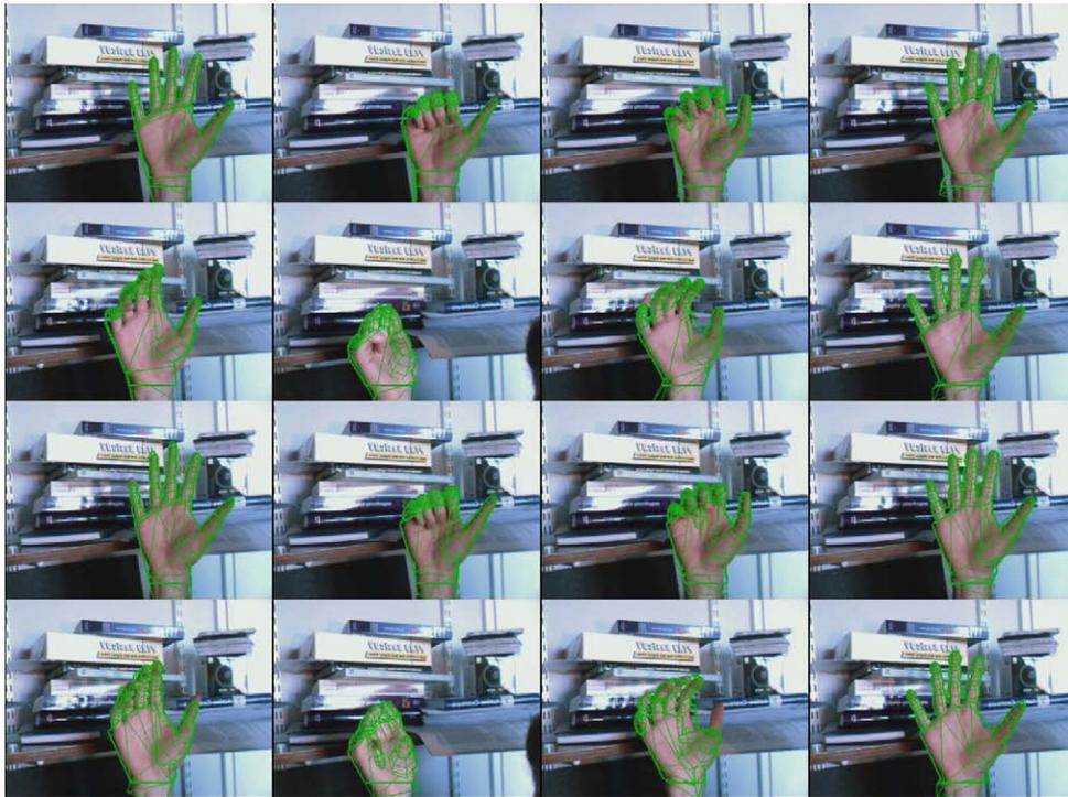
**Fig. 6.** Tracking results with a sequence provided by authors in [5] with a grasping movement of the hand, the first and second are obtained with some additional linear constraint between fingers angles. The third and fourth row are obtained without additional linear constraints.
