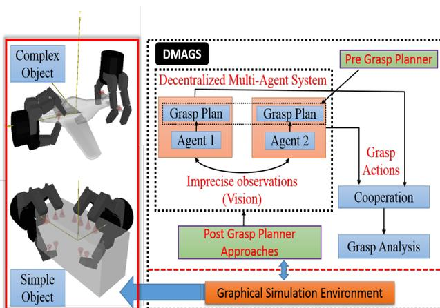
Fig. 2: Structure of Decentralized Multi-Robot Grasp System and graphical output through Graspit!.
