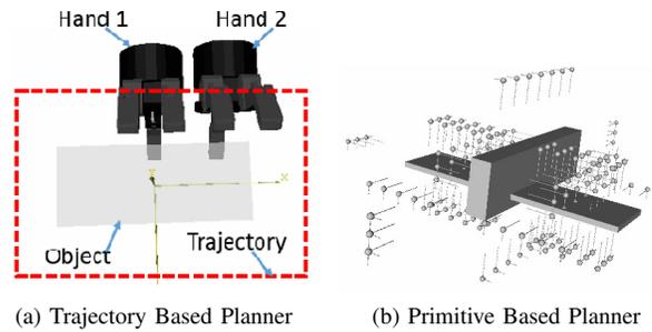
Fig. 3: Sampling-based heuristic pre planners for Box(a) and Aeroplane(b) object.
