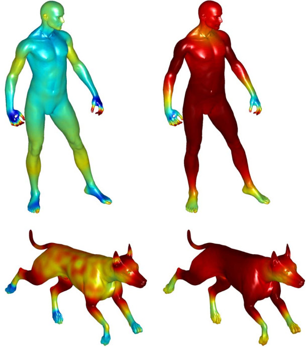
Figure 6. Normalized Euclidean distance between the descriptor at a reference point on the right hand (white dot) and descriptors computed at rest of the points of the same shape and a distinct shape (bottom row) using the SIHKS descriptor (left) and the ISC-SIHKS (right). Observe how the introduction of spatial context improves the discriminativity and localization of the descriptor.
